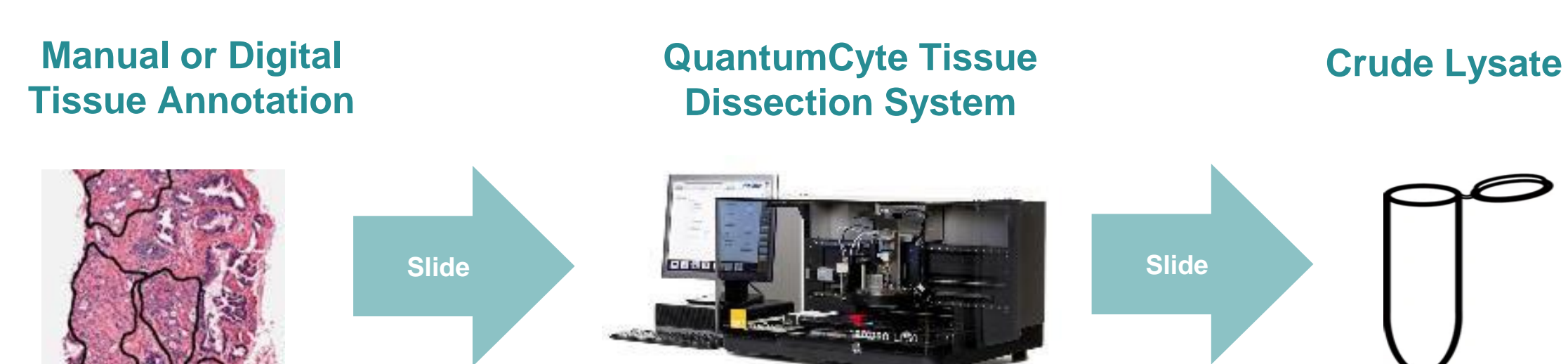
Figure 1. Quantumcyte tissue dissection system. The system is capable of extracting a crude lysate from regions of interest on a FFPE tissue slide as small as 50 microns. DNA and RNA can be purified for use in NGS analysis. Annotations (manual or automated) from scanned tissue slides guide the system to target informative ROIs.
